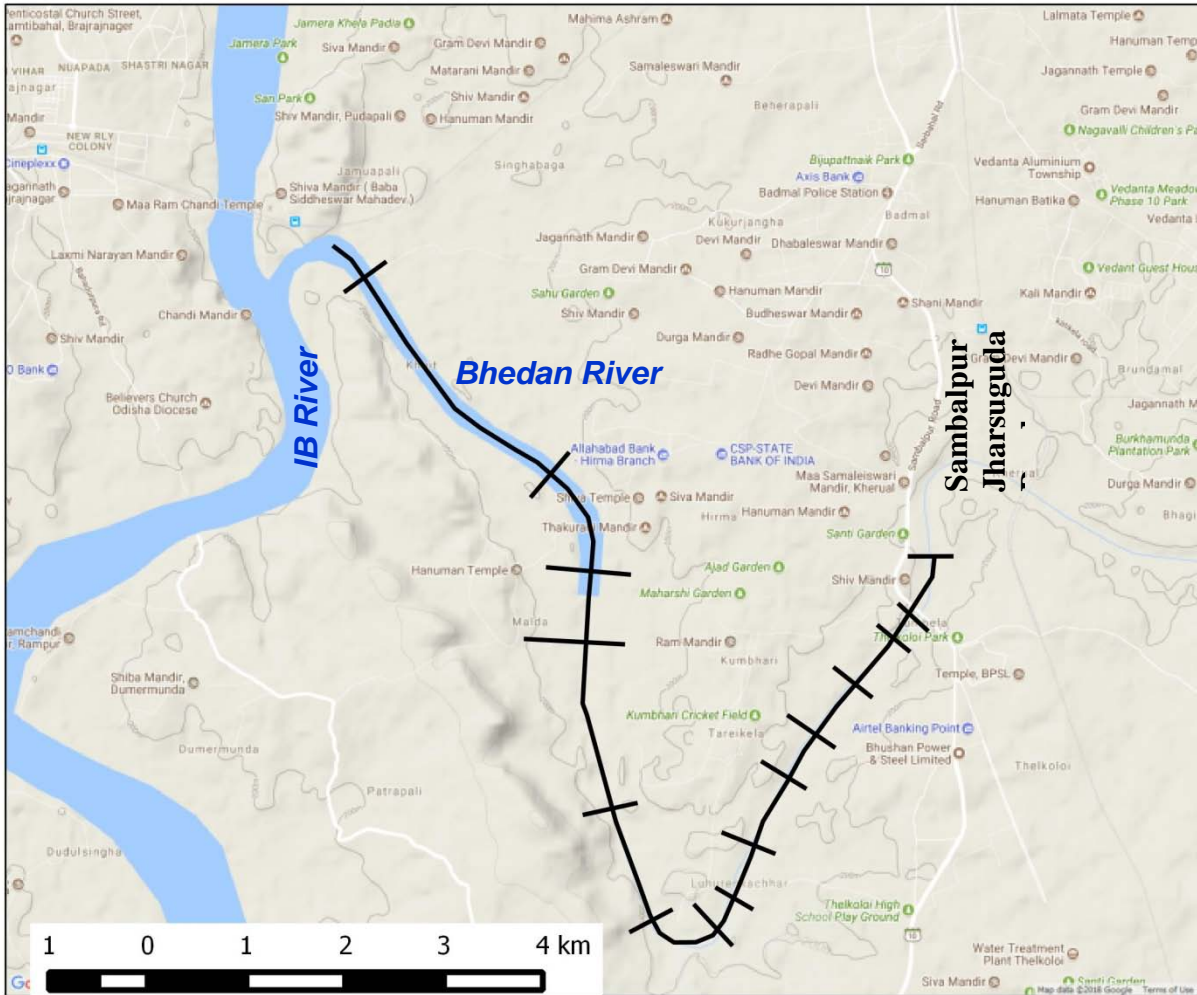
Figure 2: The stretch of river Bhedan with alignment of river cross sections survey.
