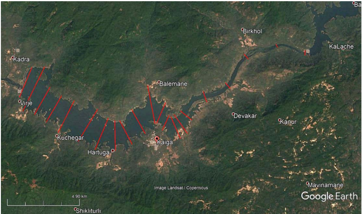
Figure 1: The stretch of Kali river downstream of Kodalasi dam for detailed river cross sections survey (red lines shows the location for survey within Kadra reservoir).
